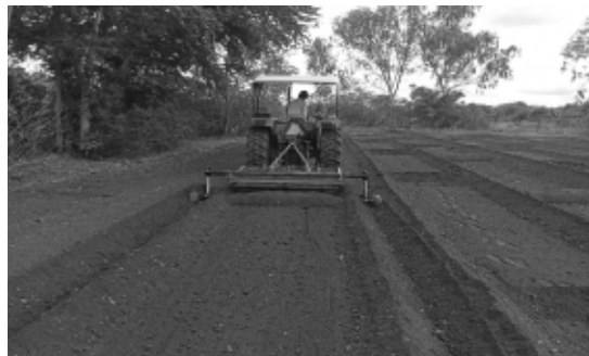
Fig. 3. Developed tractor operated ridger for basin lister
